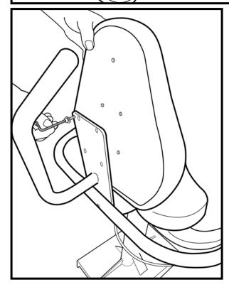
Install Upper Seat Pad with as shown with 4x M6x20mm Bolt/Washer.
