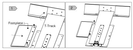
b) Mount the Left Channel over the top of the footplate dome Bolts and then slide forward. Once Channel is properly positioned, attach to T-Track using 4x M8x45 mm Bolts[16]. Repeat this procedure to install Right Footplate and Channel.
