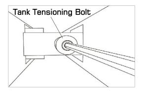
Note: Do not over tighten Tank Bolts.
