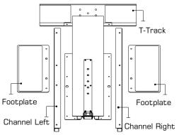
a) Tilt the T-Channel slightly to allow the footplate (with pre-installed Bolts) to slide underneath as shown.
