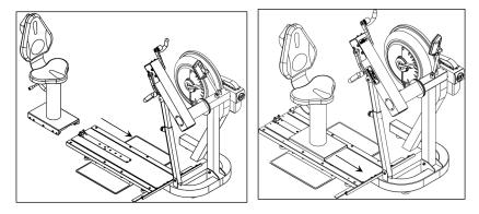
c) To remove the seat: Lift and lower the Rear Safety lock, depress the Seat Lock Release Lever and slide the seat rearward.
