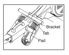
Adjust the other foot pad in the same way. Make sure to adjust both foot pads to the same position.
