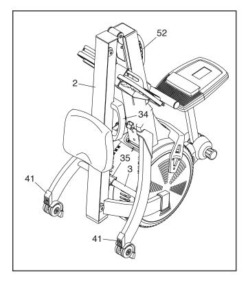
Then, hold the Rail Handle (34) and the Frame Handle (52), pull the Rail Handle outward, and lower the Rail (2) to the floor.
