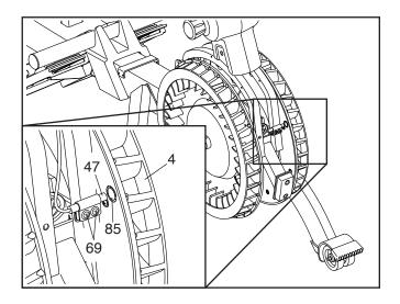
Turn the Left Fan (4) so that the Magnet (85) passes the Reed Switch (47) repeatedly. Repeat these actions until the console displays correct feedback.
