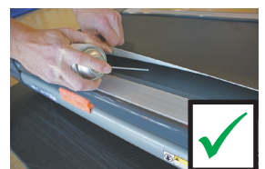
Spray evenly onto running deck
