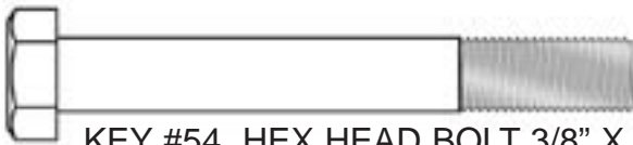
KEY #54 HEX HEAD BOLT 3/8" X 2 3/4" PARTIAL THREAD QTY. 7
