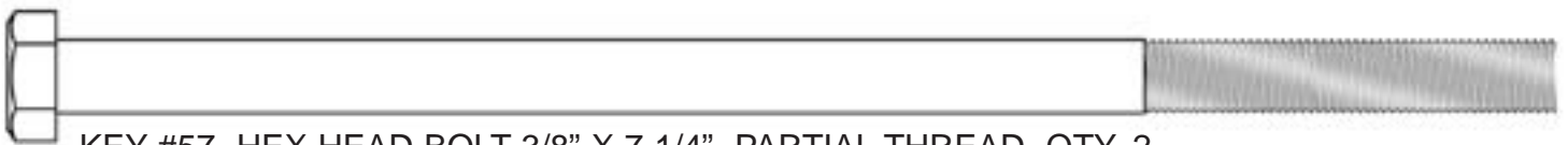
KEY #57 HEX HEAD BOLT 3/8" X 7 1/4" PARTIAL THREAD QTY. 2
