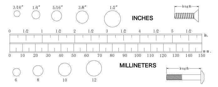
**NOTICE:** The length of all bolts and screws, except those with flat heads, is measured from below the head to the end of the bolt or screw. Flat head bolts and screws are measured from the top of the head to the end of the bolt or screw.
