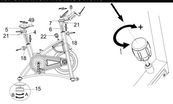
Before moving the SPIN BIKE, make sure the Handlebar (8) is tightened.
