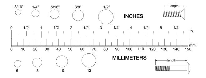
NOTICE: The length of all bolts and screws, except those with flat heads, is measured from below the head to the end of the bolt or screw. Flat head bolts and screws are measured from the top of the head to the end of the bolt
