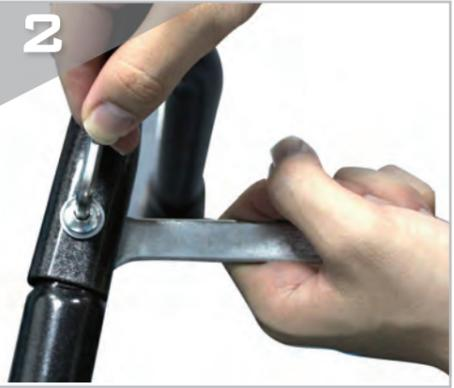
Connect now two rails with an button head screw(18),two washers(19) (one on top side and the second one on bottom side) and secure them with a nat(20)
